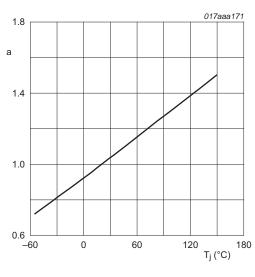
$$a = \frac{R_{DSon}}{R_{DSon(25^{\circ}C)}}$$
