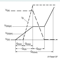
Fig 15. Gate charge waveform definitions
