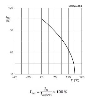
ig 2. Normalized continuous drain current as a function of junction temperature
