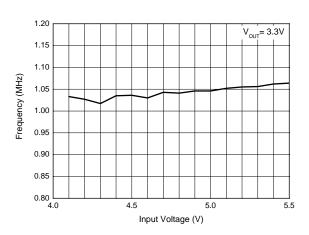
Figure 10. Frequency vs. Input Voltage
