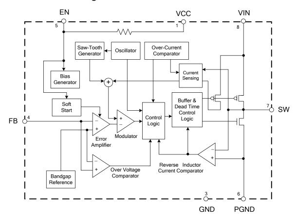
Figure 3. Functional Block Diagram of AP3435
