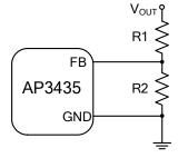
Figure 26. Setting the Output Voltage
