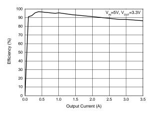
Figure 4. Efficiency vs. Output Current
