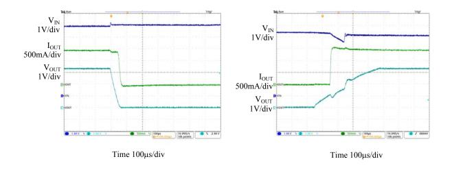
Figure 24. OVP Function (V<sub>IN</sub>=5V to 6V)
