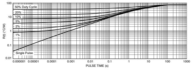
Figure 11. Thermal Response, Junction-to-Ambient
