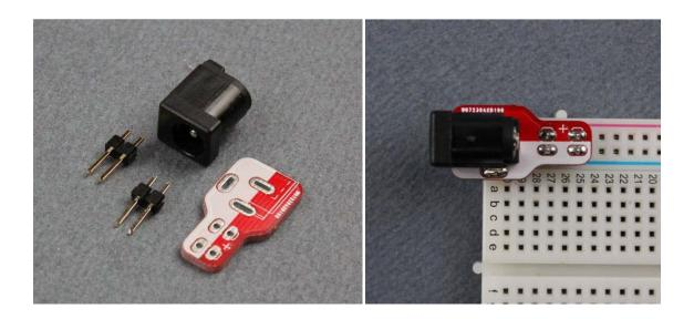
This simple little kit takes moments to solder but will make your bread-boarding life a whole lot easier for years to come. Breaking out a DC barrel jack connector it will deliver whatever power your PSU is rated for to your breadboards power rail.
