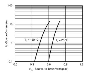
Source-Drain Diode Forward Voltage
