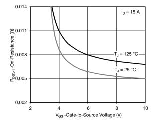
**On-Resistance vs. Gate-to-Source Voltage**
