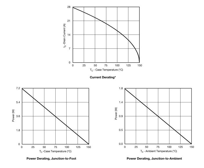
\* The power dissipation  $P_D$  is based on  $T_{J (max.)} = 150 \text{ °C}$ , using junction-to-case thermal resistance, and is more useful in settling the upper dissipation limit for cases where additional heatsinking is used. It is used to determine the current rating, when this rating falls below the package limit.
