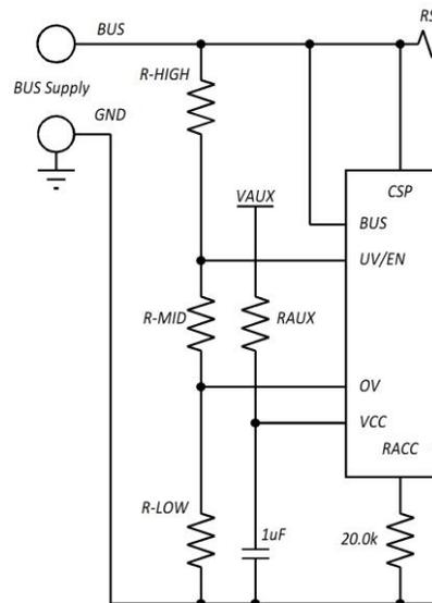
**Figure 6 - External VAUX connection for lower BUS voltages.**
