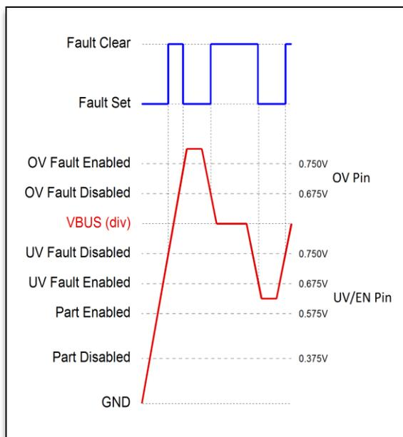
**Figure 7 - Enable, UV and OV thresholds.**
