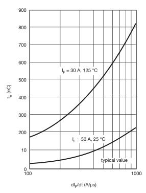
Fig. 8 - Typical Stored Charge vs. dl<sub>F</sub>/dt
