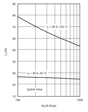
Fig. 7 - Typical Reverse Recovery Time vs. dl<sub>F</sub>/dt
