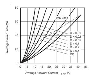
Fig. 6 - Forward Power Loss Characteristics
