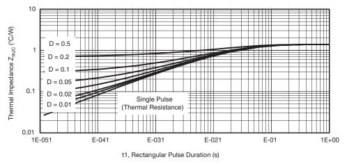
Fig. 4 - Max. Thermal Impedance Z<sub>thJC</sub> Characteristics
