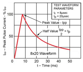
FIGURE 2 8/20 µs CURRENT IMPULSE WAVEFORM
