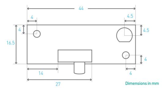
The 2 mounting holes are 3.3mm diameter.
