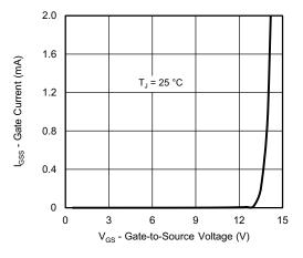
Gate-Current vs. Gate-Source Voltage
