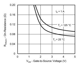
**On-Resistance vs. Gate-to-Source Voltage**
