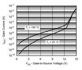
Gate-Current vs. Gate-Source Voltage
