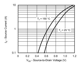
Source-Drain Diode Forward Voltage
