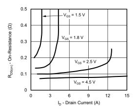
**On-Resistance vs. Drain Current and Gate Voltage**
