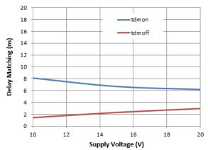
Figure 13. Delay Matching vs. Supply Voltage
