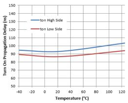
Figure 4. Turn-on Propagation Delay vs. Temperature
