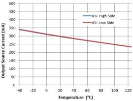
Figure 16. Output Source Current vs. Temperature
