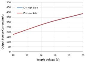
Figure 15. Output Source Current vs. Supply Voltage
