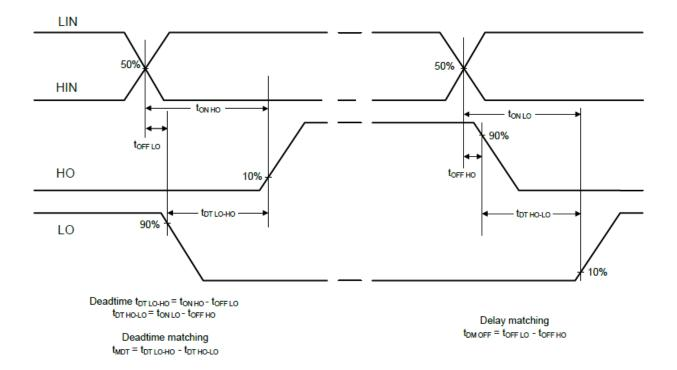
Figure 2. Switching Time Waveform Definition
