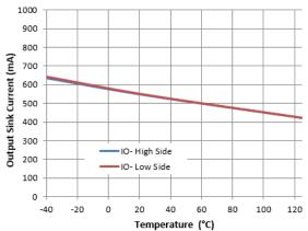
Figure 18. Output Sink Current vs. Temperature
