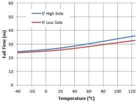
Figure 10. Fall Time vs. Temperature
