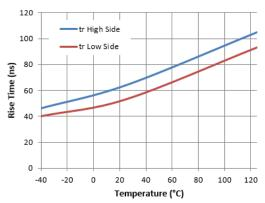
Figure 8. Rise Time vs. Temperature
