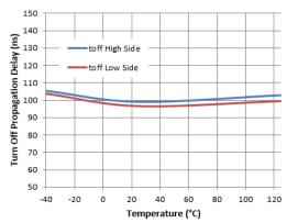
Figure 6. Turn-off Propagation Delay vs. Temperature
