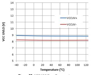
Figure 25. VCC UVLO vs. Temperature
