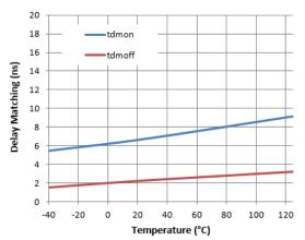
Figure 14. Delay Matching vs. Temperature
