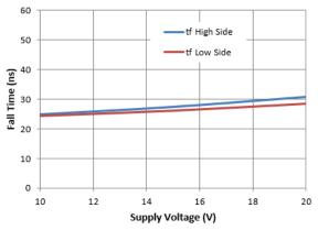
Figure 9. Fall Time vs. Supply Voltage
