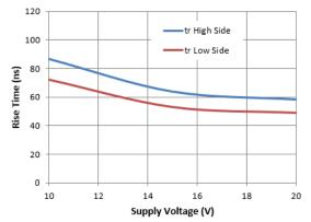
Figure 7. Rise Time vs. Supply Voltage
