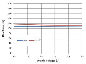
Figure 23. Deadtime vs. Supply Voltage
